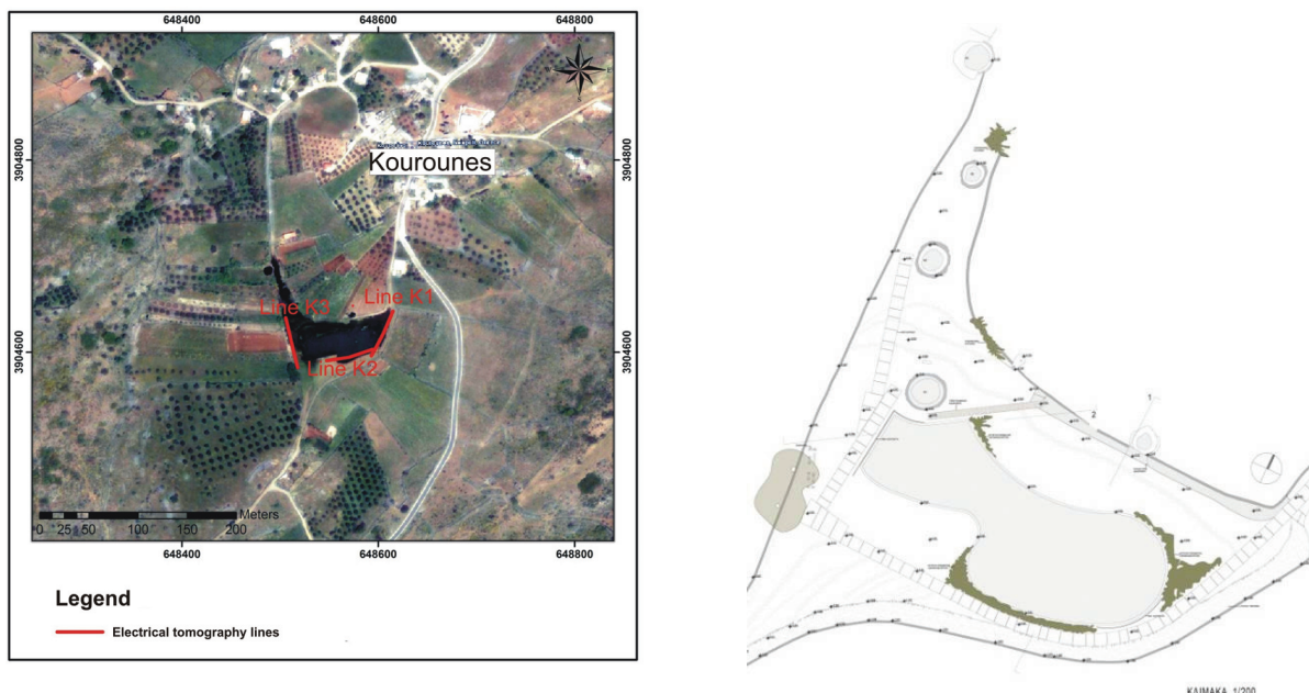
Figure 5: Satellite image of study area in Kourounes village (Google Earth) showing the position of electrical tomography lines and a proposal sketch map showing the position of the cisterns around the temporary pond
